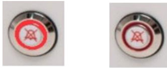
Figure 15.1 Alarm key which indicate the alarm condition
