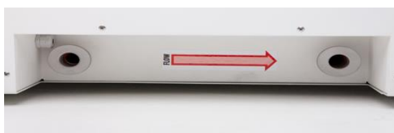
Figure 12.1 The flow arrow on the Mini MIRI® multiroom IVF incubator
